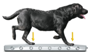
Biomechanical force platform with integrated balance. Speed between 1.7 and 2.1 m/s
